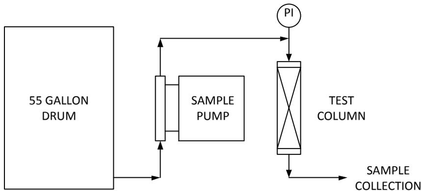
**Figure 3-1 Accelerated Column Test Flow Diagram**
